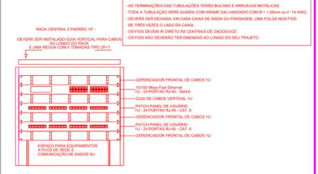
**DETALHE RACK DE 19" VISTA FRONTAL - SEM ESCALA TÍPICO**
